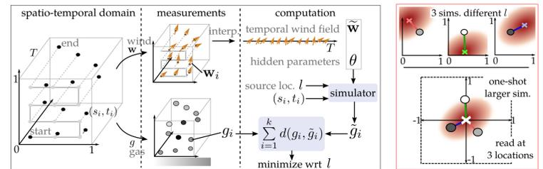
1) Wind estimations drive the simulation 2) Gas readings are compared
