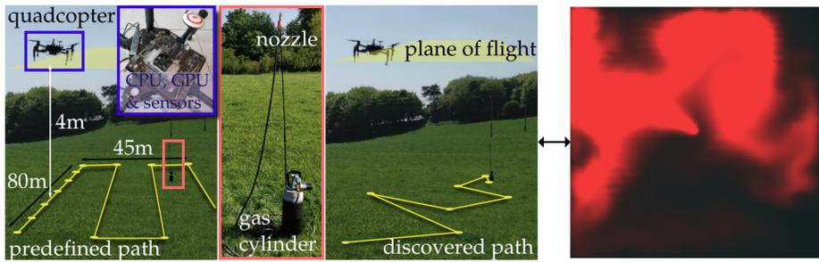
We propose a novel **gas leakage localization** algorithm by employing a **fluid simulation as a model**.
