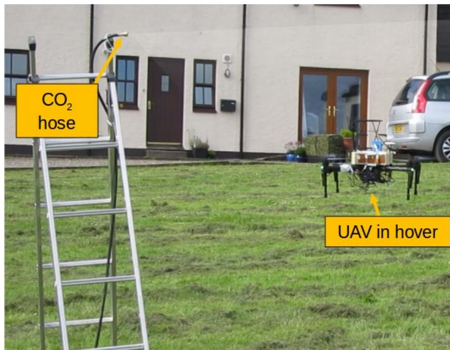
Figure 5.9: Sensing of  $CO_2$ . A successful hardware and software integration with the broadband spectrometer sensor was demonstrated. However, due to strong noise caused from the vibrations of the motors, it was not possible to get good signal and integrate the sensor within the described framework.
