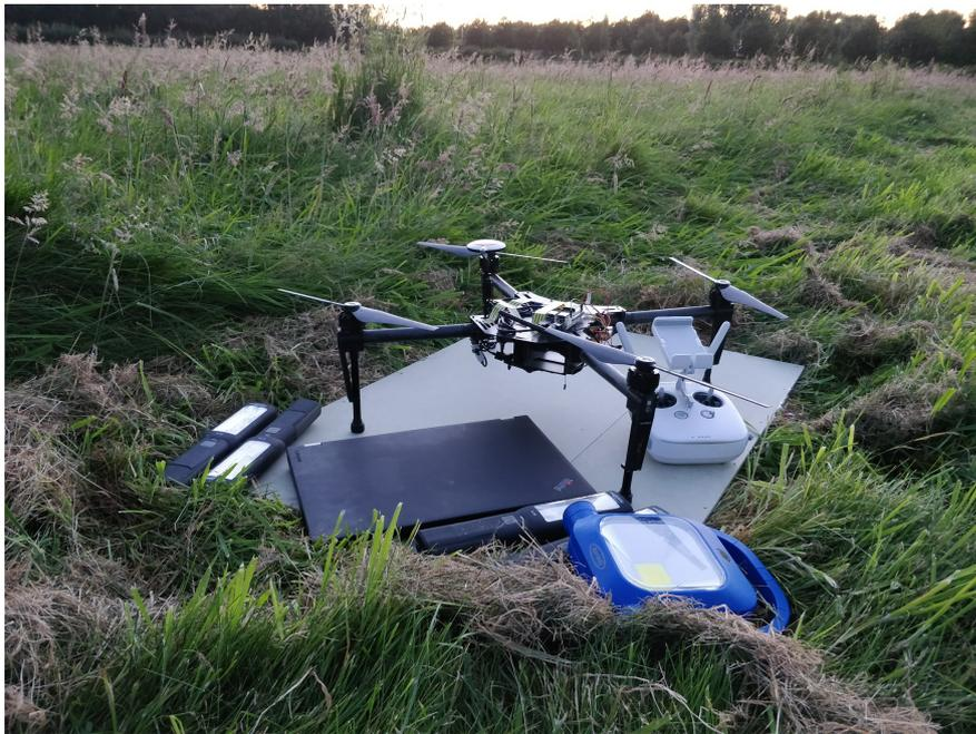
Figure 4.7: Conducting experiments during the night. When conducting light experiments, we waited until sunset and used number of industrial flash lights to generate signal for the sensor.
